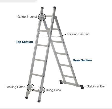
Unlock the locking catch and disengage the rung hooks. Lift the top section and open out the ladder.
