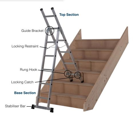
Unlock the locking catch and disengage the rung hooks. Lift the top section and open out the ladder.
