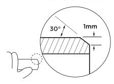
Check the tube ends are free from damage and clean, wiping away any swarf to avoid damaging the 'O' ring on tube insertion. Tube end must also be free from stickers, tape and adhesive residues.
