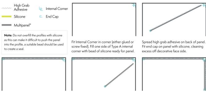
Push panel into internal corner and press against wall firmly, clean any excess silicone from corner.
