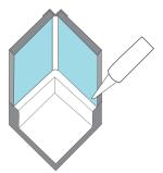
Multipanel® Seal is an all-in-one kit for sealing the bottom edge of Multipanel® at a shower tray or bath. See separate installation quide.
