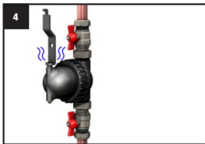
Open isolation valves. Vent out any air through the air vent then re-close using the multi tool provided.
