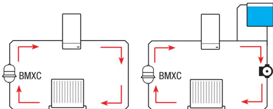
**Installation** - Always ensure the air vent points upwards
