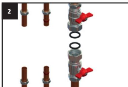
Attach isolation valves to pipework.
