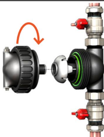
Locate the filter bowl and core into place by tightening the locking collar, making sure the air vent is positioned at the top.
