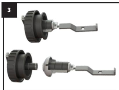
Remove the core cover with tool provided.
