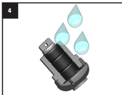
Remove any sludge or magnetite.
