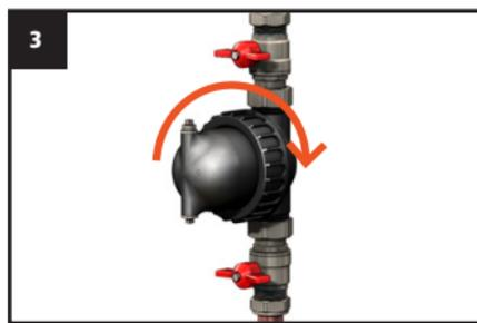
Insert the valve seals and fit the filter unit into place, tighten the nuts on the isolation valves. Ensure that the filter collar is tightened. Ensure the air vent and drain valve are closed.
