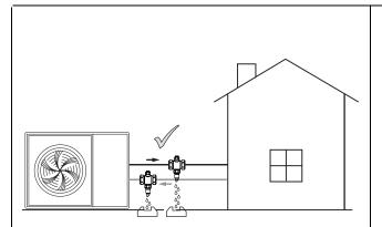
Diagram 1: The Zero antifreeze valves must be installed outdoors, closest to the heat pump, where the lowest temperatures can be reached if the heat pump is not operating.
