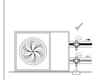
Diagram 3: In situations where the space is limited, the Zeroguard protects the anti-vacuum valve allowing the valves to be stack one above the other.
