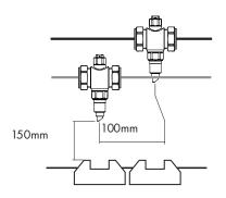
Diagram 2: We recommend 150mm clearance between the valve and the ground and at least 100mm between the valves.
